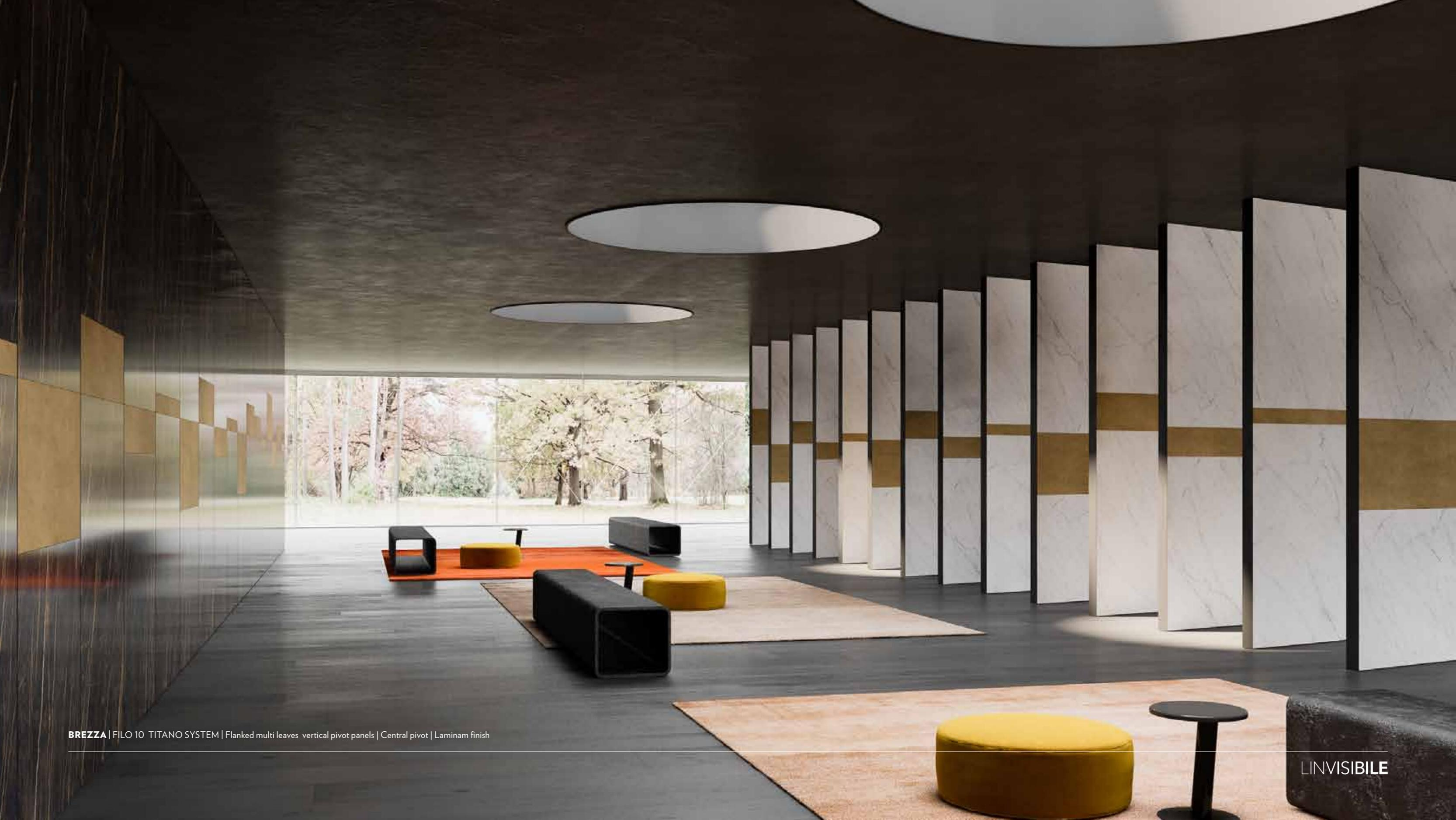
BREZZA | FILO 10 TITANO SYSTEM | Flanked multi leaves vertical pivot panels | Central pivot | Laminam finish
